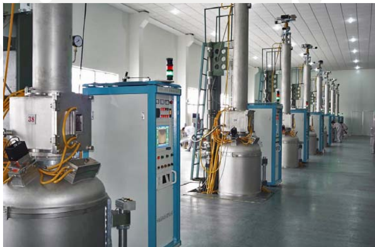
Mono crystalline furnace
